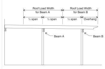
Figure 4 - Roof load width
