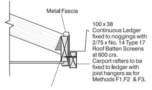
$150\,x\,50$  (140 x 45) Nogging fixed between each rafter / truss with 2/75 x 3.15 Ø nails or framing anchor each end.
